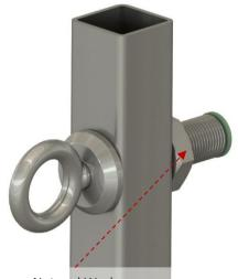
Nut and Washer (coat threads with Loctite)
